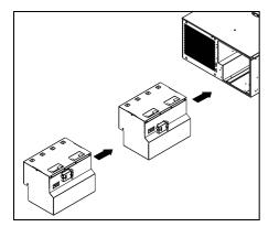
(4) Put the new battery modules back into the compartment.
